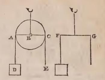
The Diameter AC, being as the beam of a ballance, of which B is the propor center. Now the parts A, and C, being equally distant from this center, therefore the power at E, must be equall to the weight at D, it being all one as if the power and the weight were fastned by two severall strings at the ends of the ballance FC.
